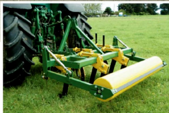
Above: The Aitchison WT6668 23-foot Easyflow Cultivator with its four rows of tines, being folded up for easy transportation.
