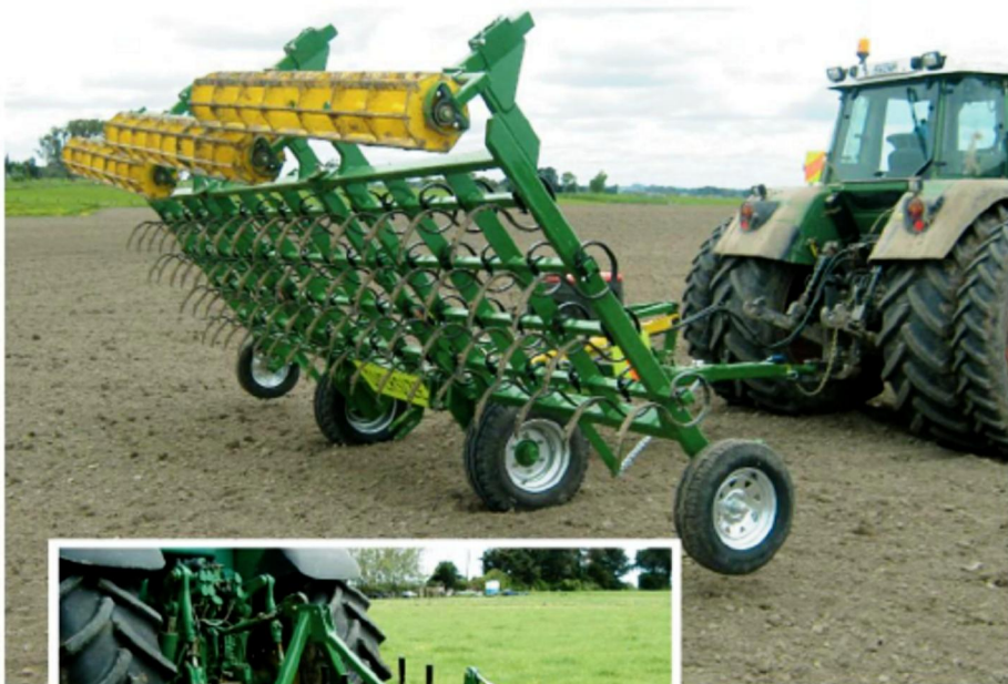
Above: The Aitchison WT6668 23-foot Easyflow Cultivator with its four rows of tines, being folded up for easy transportation.
